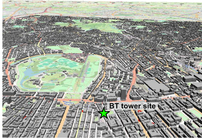
Figure 3. Bird's-eye view of buildings located in a region in the Camden borough. These building geometries are part of the static input for the PALM model. Data for the shape and height of buildings are from Ordnance Survey (Ordnance Survey (GB), 2019b, a). Background map is OpenStreetMap (OpenStreetMap contributors, 2017, ©OpenStreetMap Distributed under the Open Data Commons Open Database License (ODbL) v1.0 (for further information, please see https://www.openstreetmap.org/copyright/en )).
