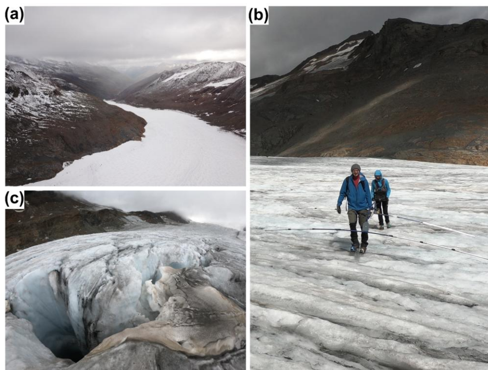
Figure A1: Field photographs from the GPR survey on Hintereisferner, Ötztal Alps, Austria, August 2023. (a) Aerial view of the GPR survey area on the lower glacier tongue, showing light snow cover following a snowfall (2 August 2023). (b) GPR survey in progress on snow-free glacier ice, showing two GPR operators carrying the Zond-xLF GPR system along a transverse profile (3 August 2023). (c) Moulin on the glacier surface, illustrating the crevassed and hydrologically active character of the lower tongue (5 August 2023).
