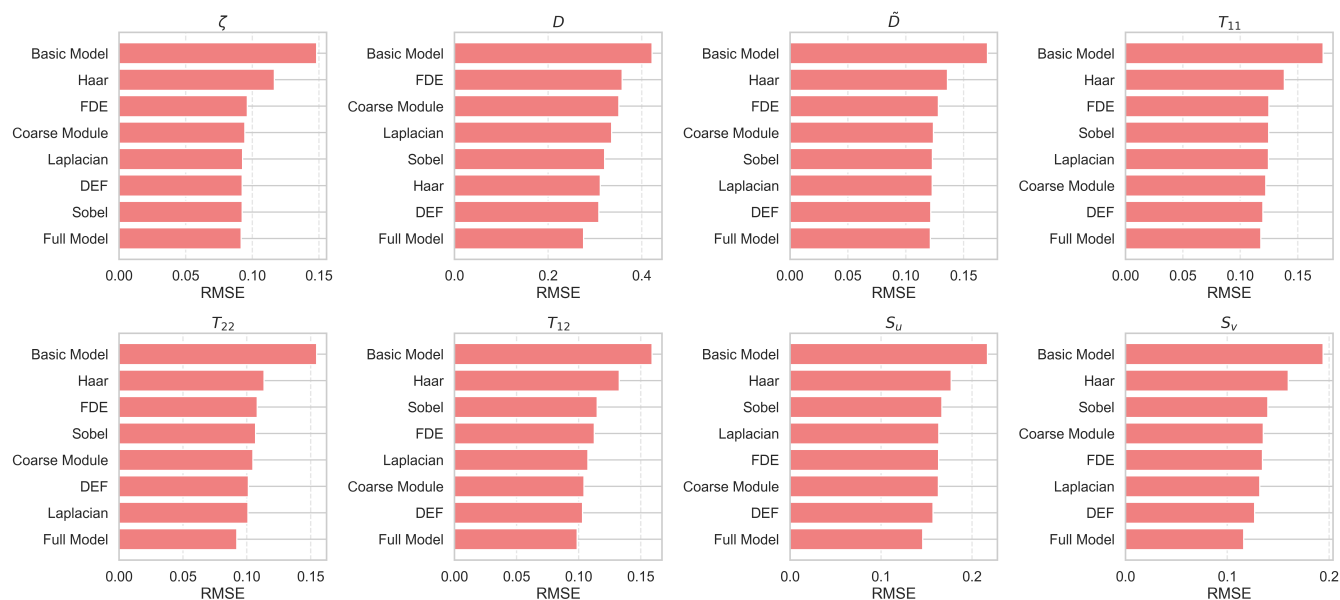
Figure 13. Per-variable normalized RMSE (lower is better) across ablation configurations. Each panel corresponds to one diagnostic— \zeta , D , \tilde{D} , T_{11} , T_{22} , T_{12} , S_u , S_v —with bars sorted in ascending order within each panel. Configurations: Basic Model (baseline), DEF, Sobel, Laplacian, Haar (wavelet), FDE, Coarse Module, Full Model. The Full Model is consistently best or near-best; the largest RMSE gains are observed for D , T_{12} , T_{22} , S_u , and S_v .
