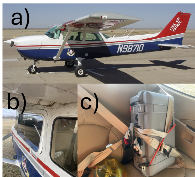
Figure 1. a) Example of a C172 Cessna used by the Civil Air Patrol (CAP) with b) an inset of the inlet tube from the LI-7810 directed out the window, and c) the LI-7810 secured in the backseat of the C172.
