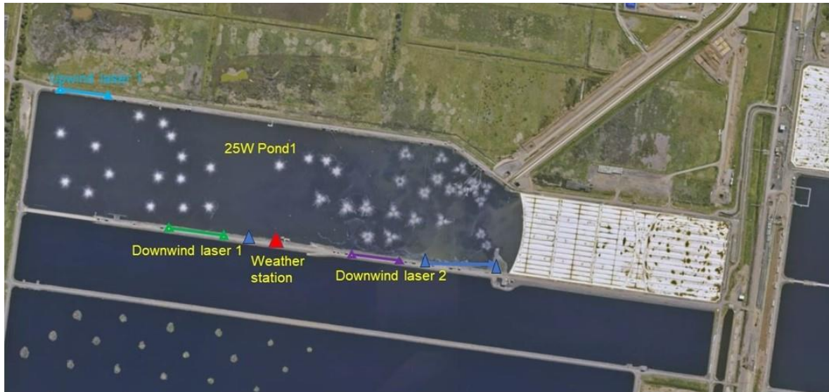
Figure 1. The layout of experimental site with one upwind open-path laser (light blue line with triangles), and two downwind open-path lasers (green and purple for summer campaign, green and blue for winter campaign). The Red triangle shows the weather station location during the summer campaign, while the dark blue triangle shows the weather station location during the winter campaign. (Source: Image @2024 Airbus, Google Earth).
