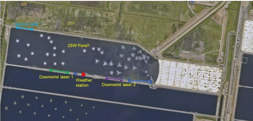
543 544 Figure 1. The layout of experimental site with one upwind open-path laser (light blue line with triangles), and 545 two downwind open-path lasers (green and purple for summer campaign, green and blue for winter campaign). 546 The Red triangle shows the weather station location during the summer campaign, while the dark blue triangle 547 shows the weather station location during the winter campaign. (Source: Image @2024 Airbus, Google Earth).
