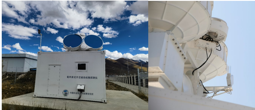
Figure 2: Field deployment of the KaW-TIR system at the Yangbajing Atmospheric Observatory, Tibetan Plateau. The right panel shows the mounting position of the thermal infrared radiometer and its relative location with respect to the radar antenna.
