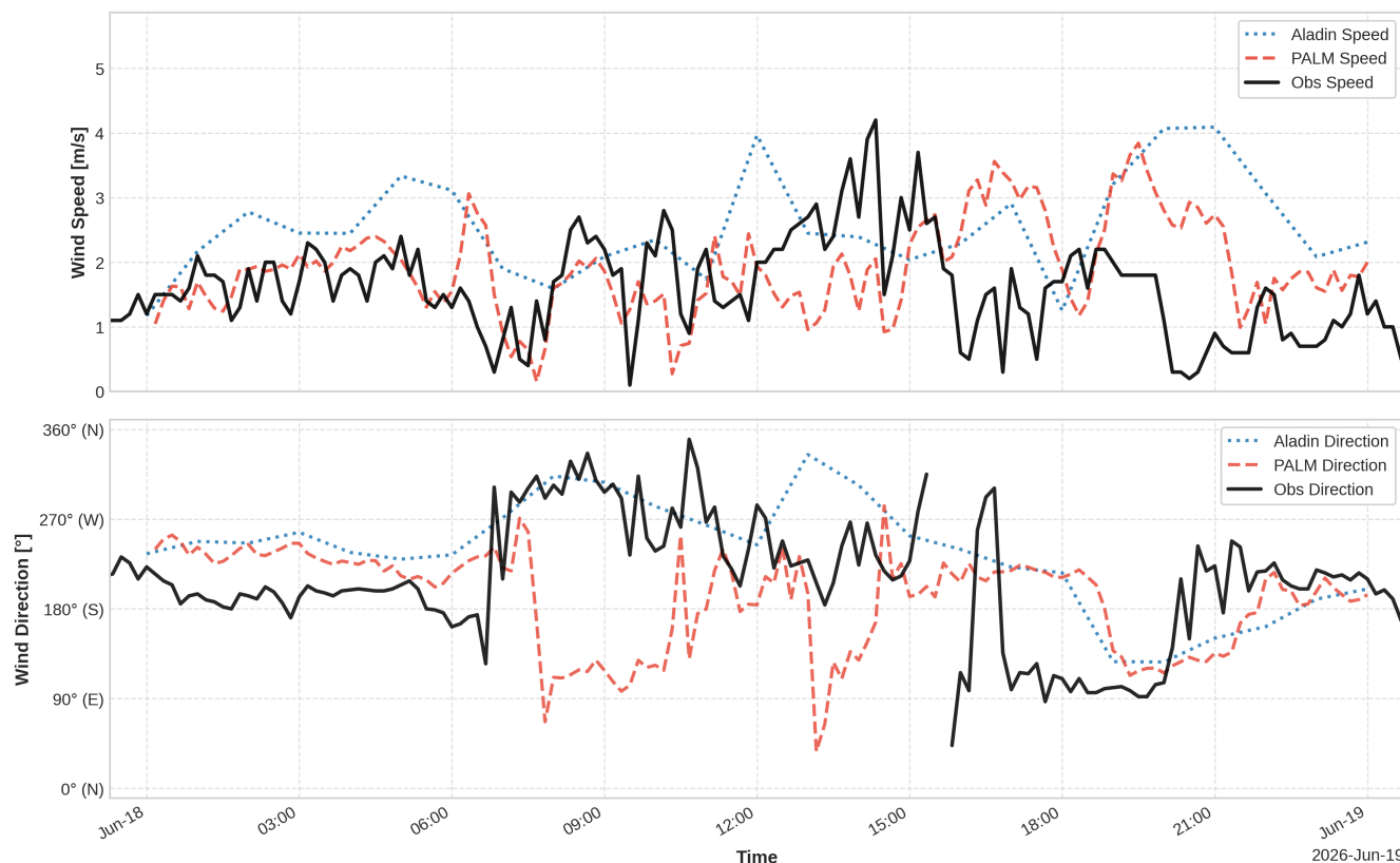
Figure A5. Comparison of the measured and modelled wind speed and direction at Prague 2-Karlov (P1PKAR01) station and the corresponding grid boxes in the models on the day of the second measurement campaign. The black line shows observations, the blue line modelled values from the ALADIN system transformed into PALM parent grid by PALM-meteo tool, and the red line values from the parent PALM domain.
