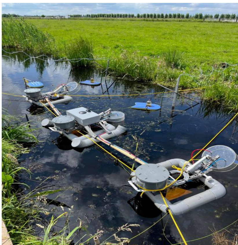
Figure 1. Impression of the automated floating chamber system. An extra floater—mounted on top of the centre floater—carries the box containing the multiplexer and its components (Fig. 2) as well as a light sensor (measuring photosynthetically active radiation) mounted on top of the box.
