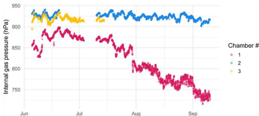
Figure S6 Pressure measured within the plumbing system by the sensor located near the inlet of the CO 2 sensor (Fig. 2). The colours represent each of the different flux chambers.
