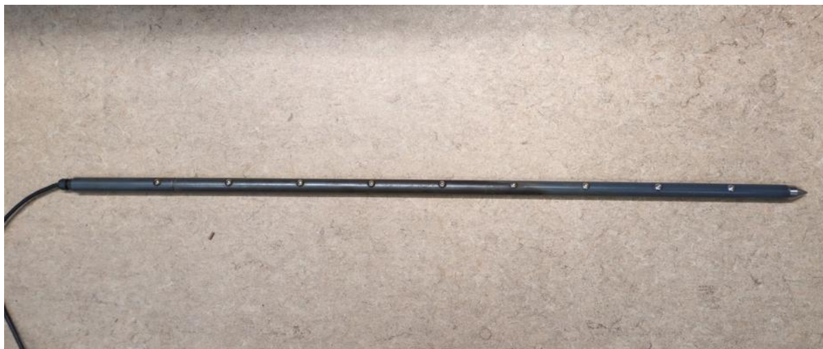
20 Figure S3 Photo of the probe used to measure the temperature profile (10 cm intervals) in water and sediment. The probe can be connected to the chamber system to have its data log integrated with that of the other sensors.
