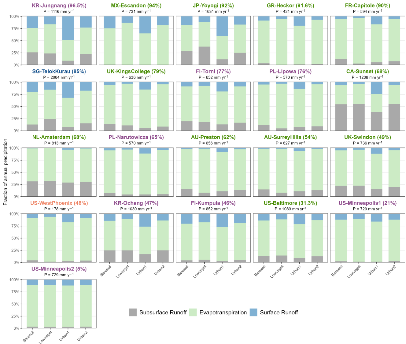
Figure 67: Mean annual partitioning of precipitation into evapotranspiration, surface runoff, and subsurface runoff for each site and simulation. Each stacked bar represents the three components as fractions of mean annual precipitation. Mean annual precipitation is indicated above each panel. Mean annual water budget by station and by simulation. Simulated years depend on station (12-16 years). Titles' colours indicate the climate of station: green for Temperate, purple for Continental, orange for Dry and blue for Tropical. Percentage in title indicates the urban coverage around the station.
