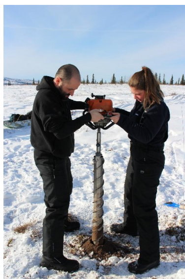
Figure 4: Winter field access to supra-permafrost taliks using motorized drilling systems at Eight Mile Lake, Alaska (USA). Drilling through the seasonally frozen active layer is required to access unfrozen talik soils, where pore waters remain liquid year-round beneath the frozen surface. Talik soils are collected and placed into plastic bags, using insulated processing to prevent rapid freezing upon exposure and pore waters are subsequently extracted using Rhizon samplers. This approach enables direct biogeochemical sampling during the winter months, the season when taliks are most clearly distinguished from surrounding frozen ground. The authors have obtained written consent to publish the image.
