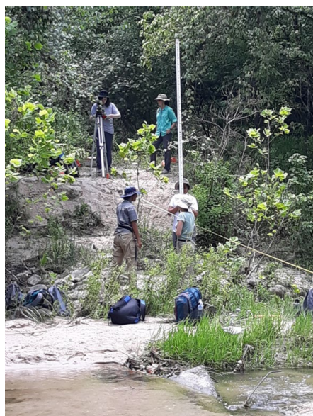
Figure 2. GET TX participants using survey equipment to measure a stream profile at SHSU's Pineywoods Environmental Research Laboratory.
