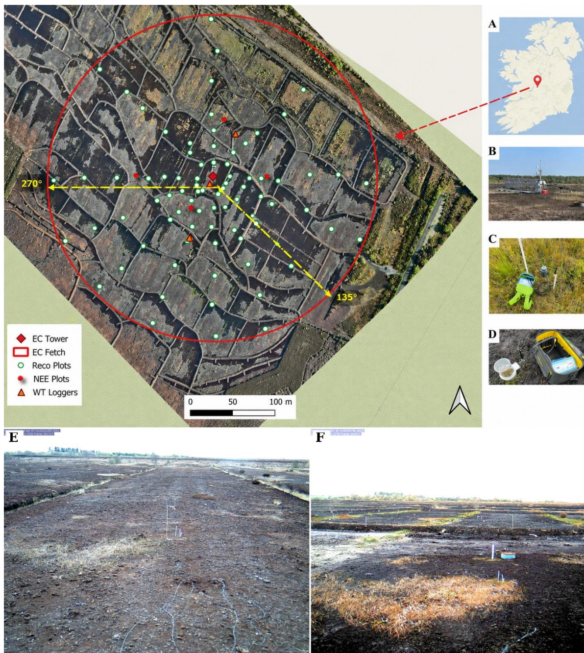
Fig. 1. Study site and field measurements at All Saints Bog, Ireland: (a) Location of All Saints Bog within Ireland and orthomosaic aerial image of the rewetted peatland showing the eddy covariance (EC) footprint, EC tower, FC measurement plots, and water-table (WT) logger locations; (b) EC tower installed within the rewetted cutaway bog; (c) Dark chamber used for ecosystem respiration ( R_{eco} ) measurements; (d) Transparent chamber used for net ecosystem exchange (NEE) measurements; (e) Site conditions before rewetting in April 2021; (f) Site conditions after rewetting in September 2024.
