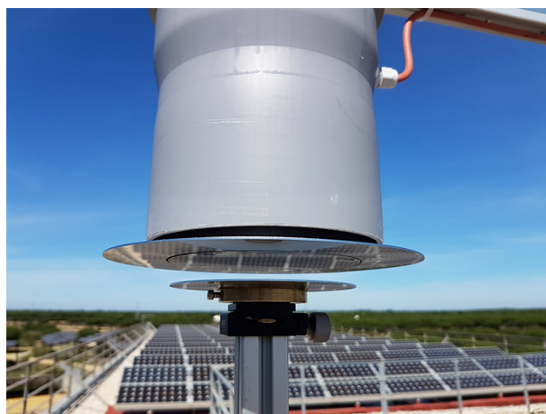
Figure 2. Dry deposition collector. In the top part is an actuator, which lowers the outermost section in case of rain to protect the lower plate of the collector from rain. Rain is detected by an infrared rain sensor.
