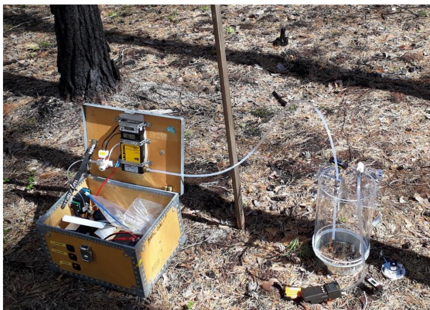
155 Figure 2. In-situ BVOC measurement setup. A transparent chamber was placed on the forest floor and connected to a pump box supplying purified purge air free of BVOCs and ozone. Air from the chamber was drawn through adsorbent tubes using portable pumps to collect BVOCs emitted from the forest floor.
