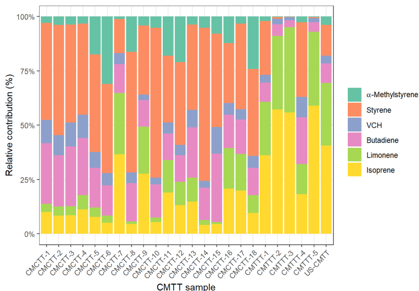
255 260 Figure 2. Relative contribution of the selected six markers (individual signal intensity relative to the sum of the intensities of all six peaks) for all cryo-milled tire tread samples. CMCTT-1 to 18 are samples from used tires for passenger cars, and CMCTT- 1 to 5 are samples from used truck/bus tires, and US-CMTT is a mixture of car, truck and bus tires.
