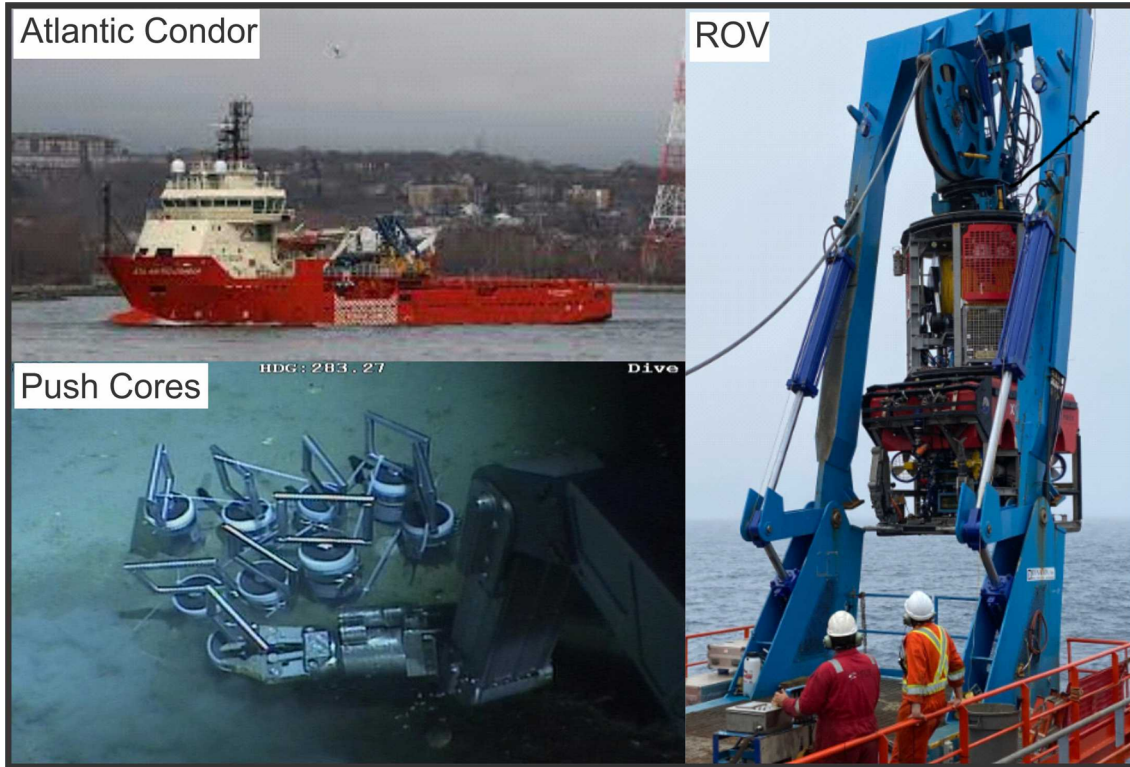
Figure S6: Push core sampling techniques employed during the 2021 expedition.
