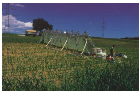
Figure 2 Transportable rainfall simulator (Scherer et al. 2012).
