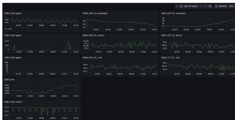
300 301 Figure 4. Time series of a 12 hour continuous observation acquired by the SMART- 302 ASF system and visualized using Grafana, showing synchronized measurements of 303 chamber gas concentrations, temperature, humidity, soil parameters, atmospheric 304 pressure, and system voltage. Data were recorded at 10 second intervals and transmitted 305 in real time to cloud and laboratory servers.
