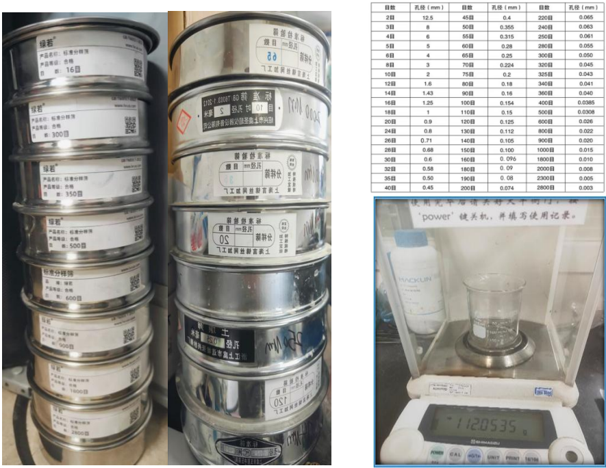
Fig. S2. Sieving and weighing of source area soils and suspended sediment samples.
