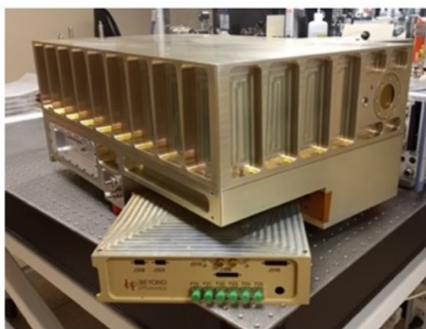
357 Figure 4: The AWP Local Electronics Module partially removed from the HPM.
