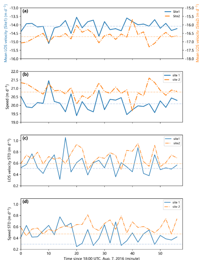
Figure 6 Time series of 29 interferometric pairs with 2-minute temporal interval at two sites. Statistical analysis is performed on data at point M in Figure 1 to obtain LOS velocity mean values (a) and standard deviations (c) for each site; subsequently, NL-GWR is applied to interferometric data from each small-time segment separately, with other settings consistent with the main text, to obtain Speed mean values (b) and standard deviations (d) within the same region. Solid lines represent results from small time segments, while dashed lines represent temporal averages of the 29 datasets, i.e., the results using the data employed in the main text
