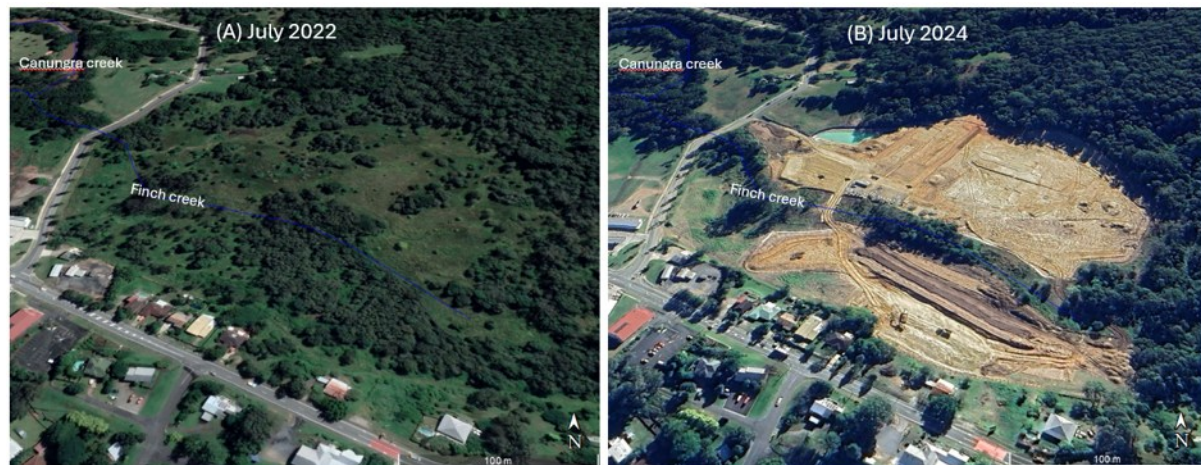
Figure S7: land clearing for urban development exposing subsoils with limited runoff management to the intermittent Finch Creek during the time of the Cyclone Alfred event in Canungra township (-28.016426, 153.167009)
