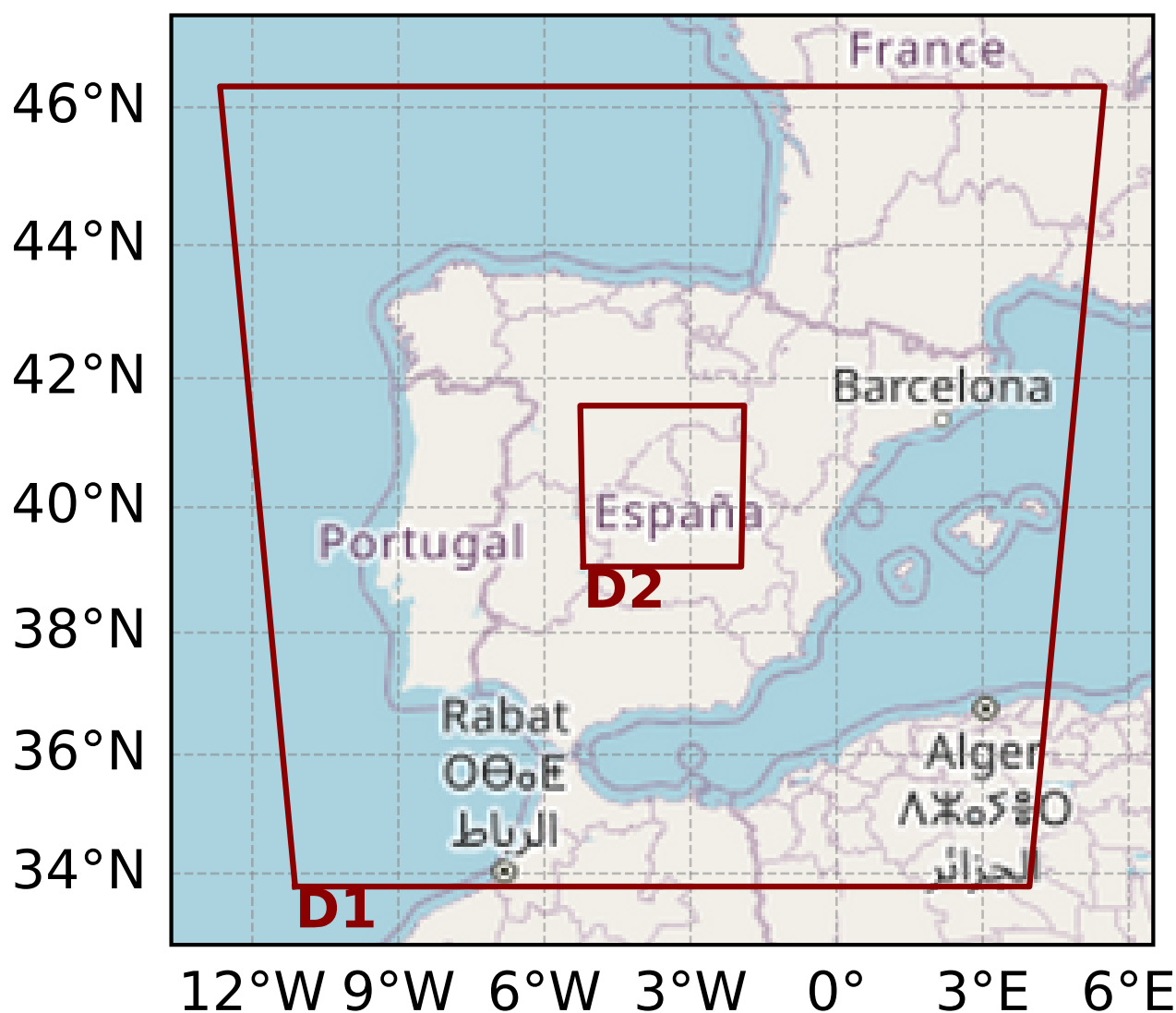
Figure 1. Illustration of the size and location of the domains used in the WRF setup.
