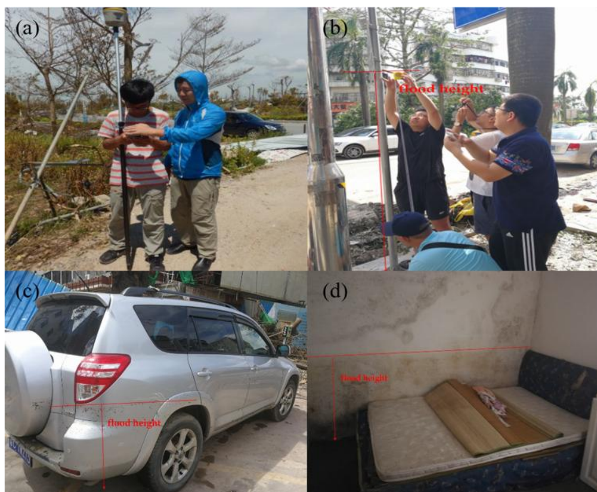
Figure 4. Example of topographic tools and techniques used for flood range measure. (a) and (b) location of flood range using RTK, (c) and (d) determination of flood height or water depth during flood using a measure tape.
