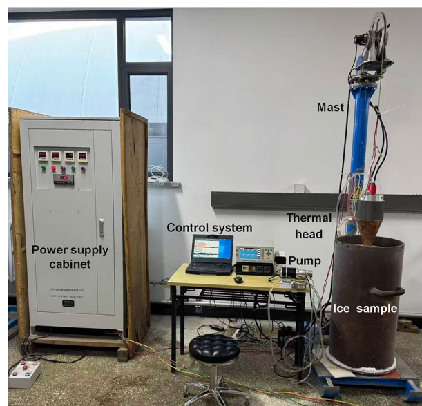
Figure 11. Test stand of the updated RECAS thermal head
