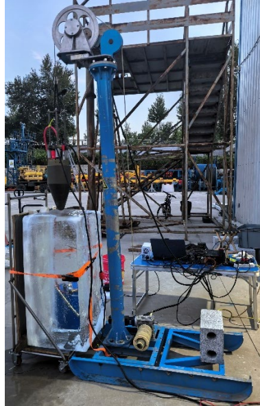
Figure S2 Test of updated RECAS thermal head with transparent ice block
