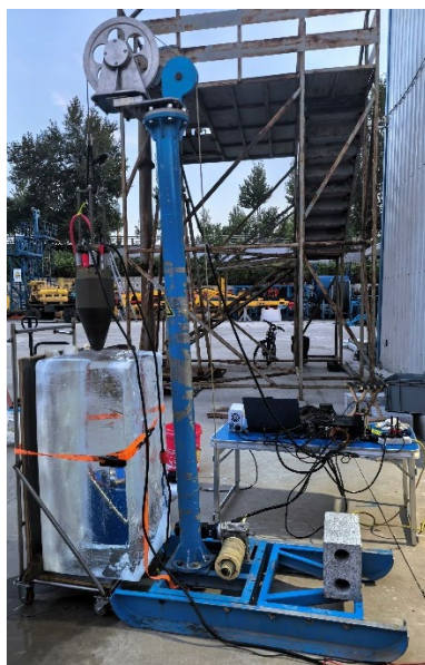
Figure S1 Test of updated RECAS thermal head with transparent ice block
