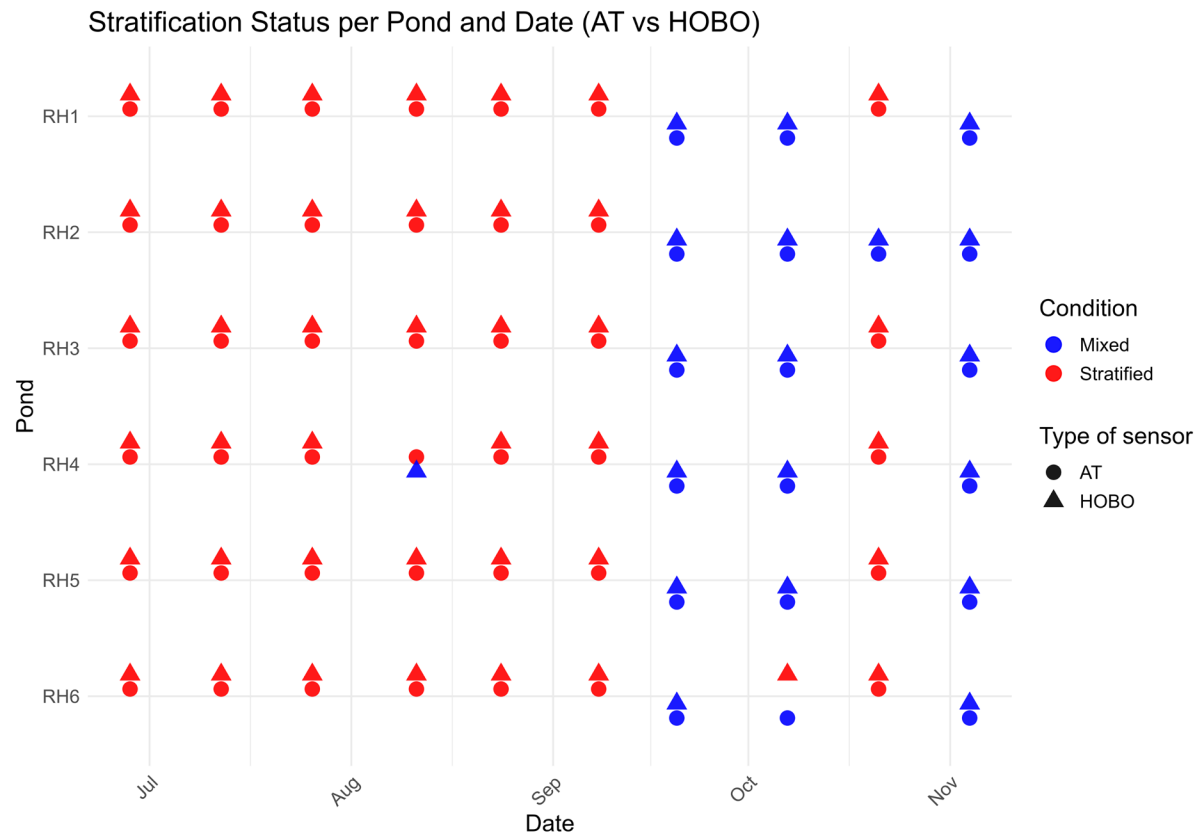
Figure S2 Comparison of mixed (in blue) and stratified (in red) patterns recorded by Aqua TROLL sensor (circles) and HOBO loggers (triangles). The measurements represent the data from the six ponds (noted RH1-6) measured from 28 June to 4 November 2021
