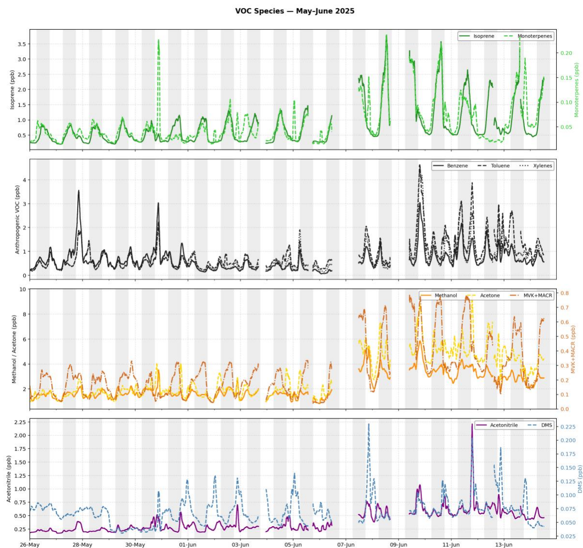
Figure S11. Time series of individual VOC species at 1 min resolution during the campaign (26 May–14 June 2025): (a) biogenic VOCs, isoprene (left axis) and monoterpenes (right axis, dashed line); (b) anthropogenic VOCs, benzene, toluene, and xylenes (BTX), distinguished by line style; (c) oxygenated VOCs, methanol and acetone (left axis) and MVK + MACR (right axis, dash-dot line); and (d) acetonitrile (left axis) and DMS (right axis, dashed line). All concentrations are in ppb. Lines show 105 min centred rolling means. Grey shading indicates daytime hours (06:00–18:00 IST). Gaps correspond to instrument downtime or data-quality screening.
