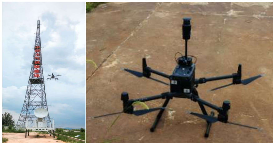
Figure 1. (a) Snap shot of the meteorological tower deployed at the Xingtai Field Scientific Experiment Base; (b) The multi-rotor UAV platform and integrated airborne meteorological payload used for field observations in this study.
