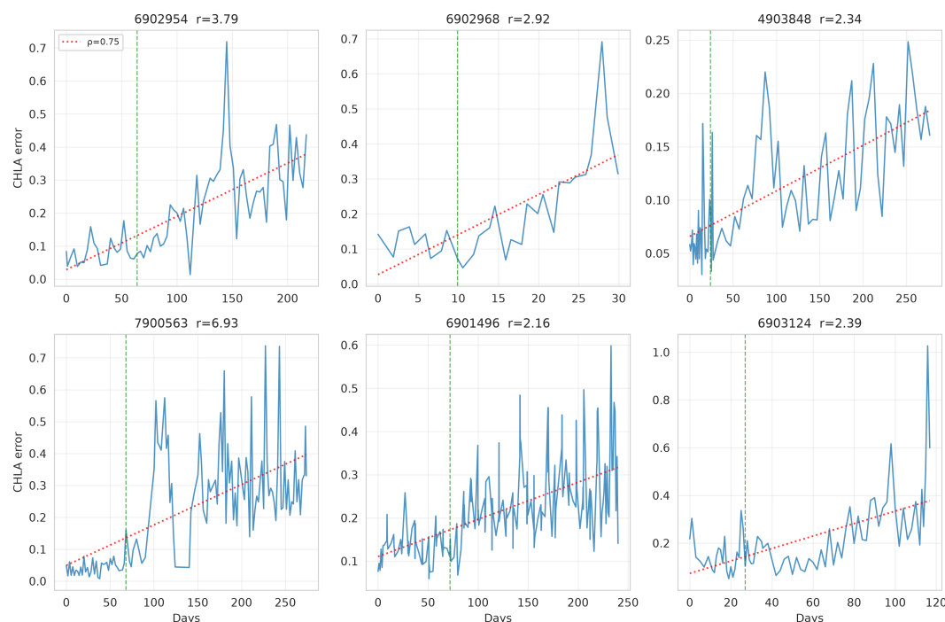
Figure 3. CHLA reconstruction error over deployment time for the six floats with strongest drift detection ( \rho > 0.5 ). Green dashed line: clean/evaluation split (30%). Red dotted line: linear trend. All detecting floats show a clear monotonic increase, consistent with progressive biofouling.
