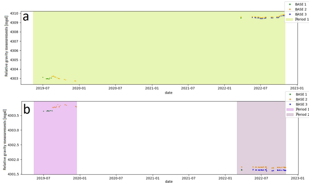
745 Figure B4: Result of intra-period drift correction after determining a one-period (a) and two-periods (b) drift function.
