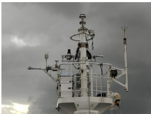
Figure S2: TSP sampler ECHO PUF together with radiometric measurements on the atmospheric mast of ATLANTE.
