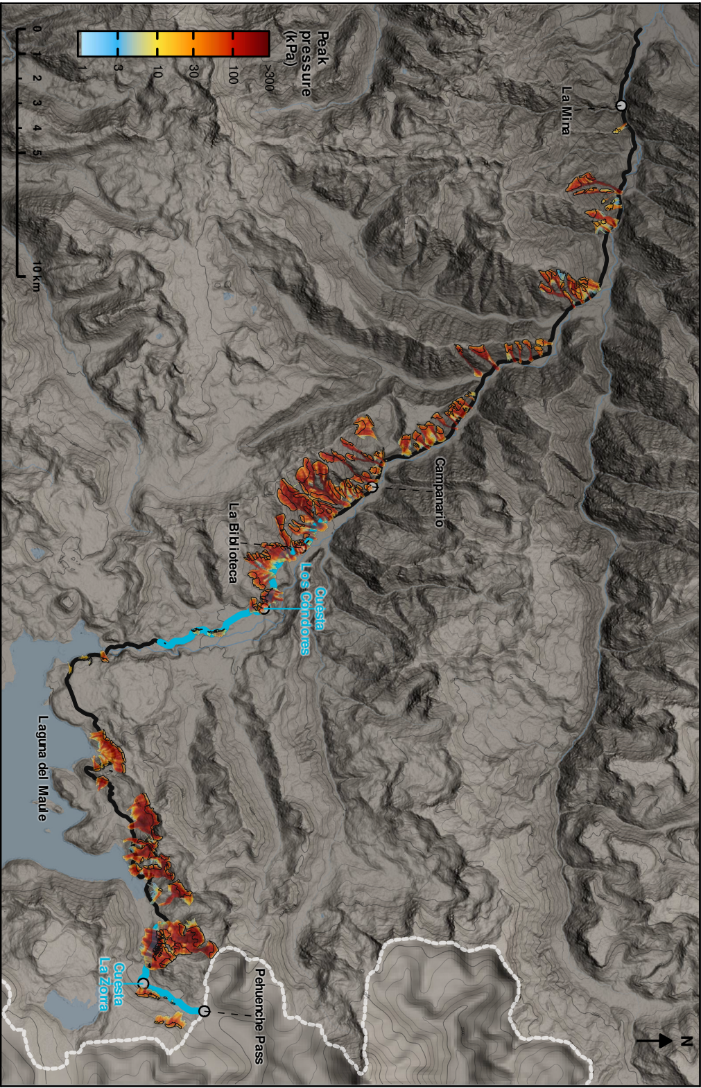
Figure 4. Avalanche intensity map for Route 115-CH (Severe scenario, T_{hs} = 30 yr): maximum peak pressure envelope across all 208 simulated paths (color scale saturated at 300 kPa). Release areas are outlined in black.
