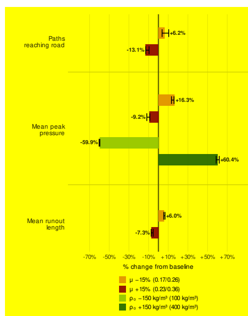
Figure 6. Sensitivity of corridor-scale exposure metrics to friction ( \mu \pm 15\% ) and release density ( \rho_0 \pm 150 \text{ kg m}^{-3} ), as percentage change from the baseline under the Severe scenario (whiskers span the T10–T100 range). Metrics: path count, mean peak pressure, mean runout.
