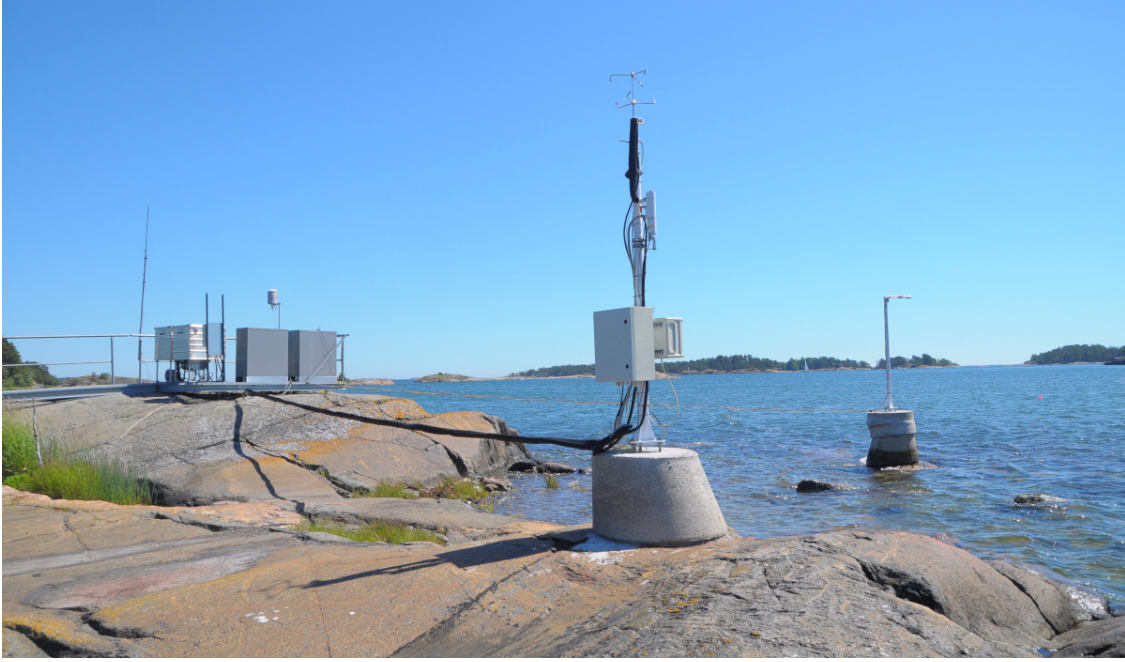
Figure S1: Photograph of the eddy covariance site, looking southeast. The EC tower is in the middle of the photograph. The mast with the radiometer is standing on the concrete base in the sea. Cabinets for the computers as well as the temperature ( T ), relative humidity ( RH ) and radiation sensors are located at the highest point of the islet.
