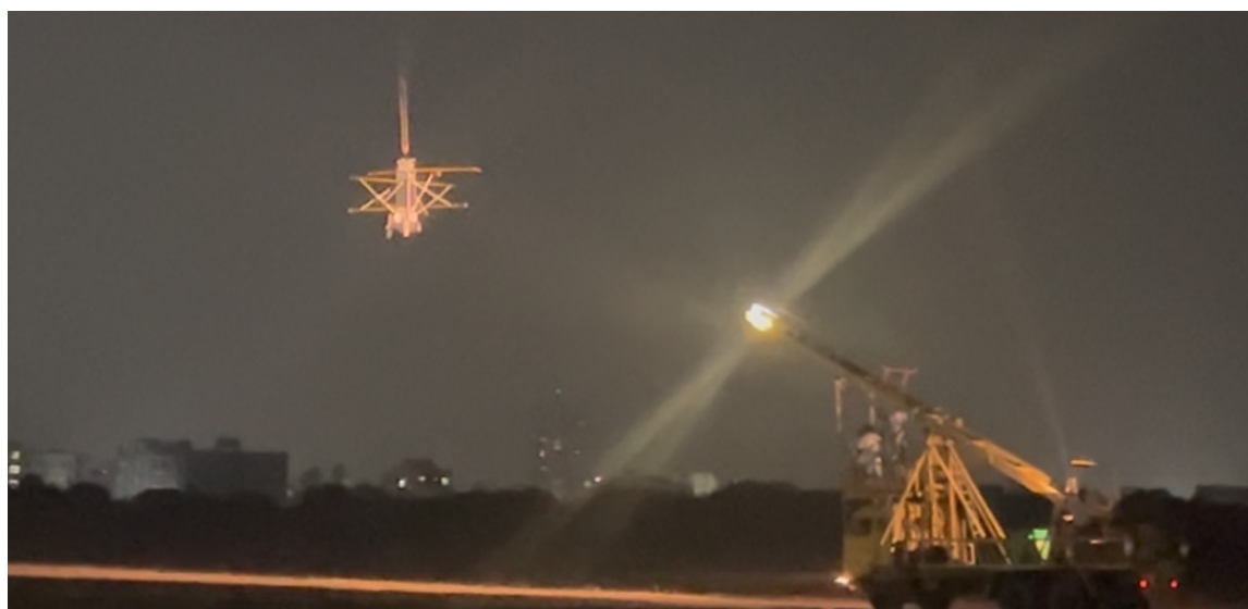
Figure 3: Payload release from the launch vehicle. The gondola and extended booms are visible at the top left, while the balloon itself is outside the frame.
