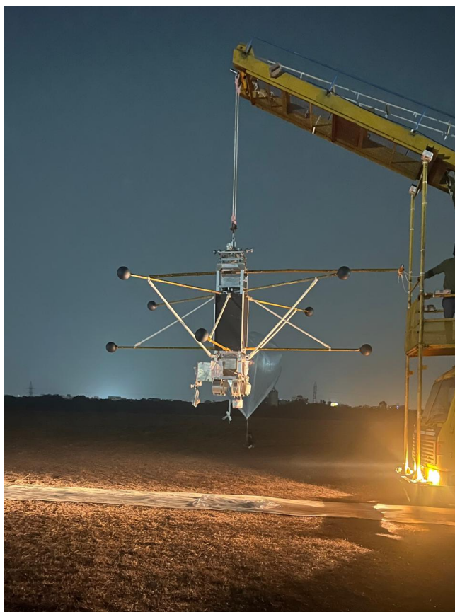
Figure 2: The BEENS-2 payload showing the gondola equipped with four pairs of electric field probes. This picture was captured just prior to launch.
