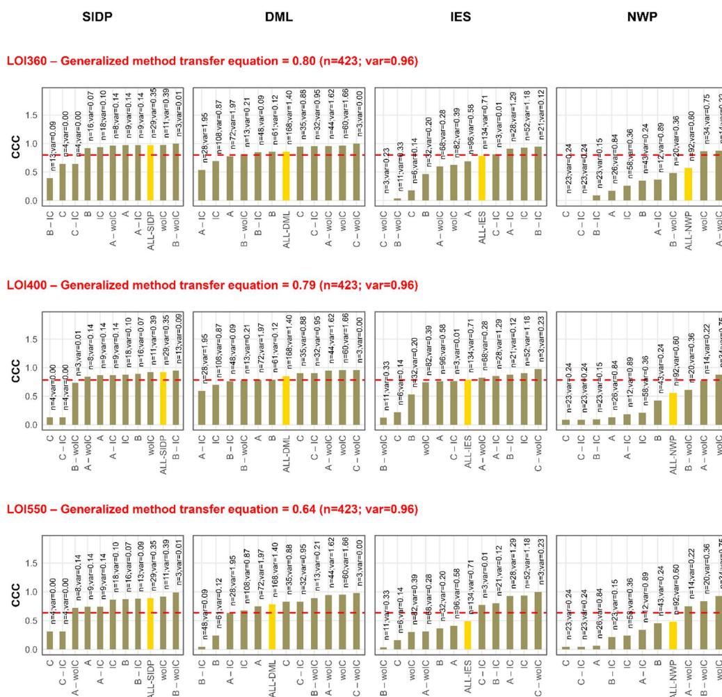
Figure 8: Comparison of CCC values between generalized and localized LOI-SOC method transfer equations for LOI360, LOI400, and LOI550 across the four landform regions evaluated. The red dashed line represents the CCC of the generalized method transfer equation using all samples (ALL) from this study, which serves as the reference for evaluation. Bars exceeding this line represent localized method transfer equations with improved concordance relative to the generalized method transfer equation. Yellow bars correspond to the method transfer equations localized to the respective landform regions only (i.e., models built using all samples within each landform region), while olive bars represent method transfer equations created by segmenting the data to more specific factors (IC content, horizon, or their combinations). Segmentations involving samples with IC are labeled “IC”, whereas segmentations involving samples without IC are labeled “woIC”. Horizon-
