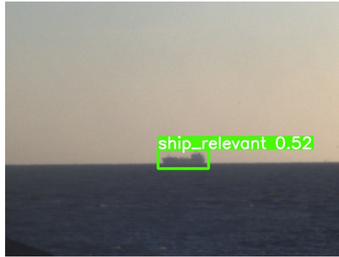
Figure 4. The YOLO image recognition software is trained on a database of ship images. The green box indicates where the algorithm recognises a ship and denotes the confidence level of the recognition. It recognises ships in various conditions, at large distance and low contrast.
