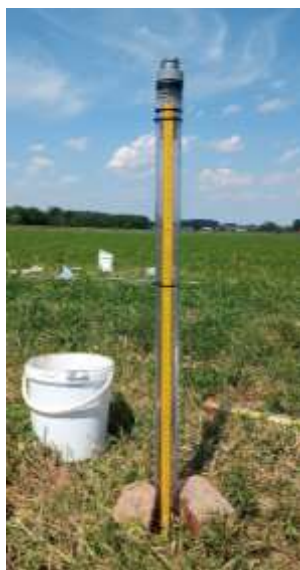
Figure A1: Field set up for the permeability test. A cylinder preably filled with water is inserted into a borehole (15 cm diameter, around 20 cm in depth) and the water flow rate is measured to calculate K_{sat} .
