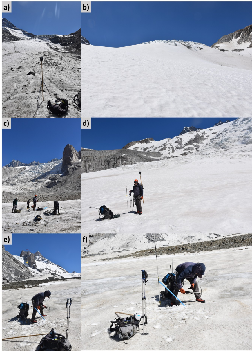
Figure S10. Field survey and stake installation on Universidad Glacier, 2024–2025 GNSS campaign. (a) GNSS receiver on tripod set up on stable ground for base-station/differential positioning, with the glacier tongue and icefall in the background. (b) View across the upper glacier surface toward the icefall. (c) Field team preparing equipment on the glacier surface, with surrounding peaks including the prominent rock tower visible in the background. (d) A team member with GNSS rover pole and ice axe standing beside a marked ablation stake location on the glacier surface. (e, f) Installation of an ablation stake: drilling into the ice with an ice axe and hand auger and inserting the stake, with the GNSS rover pole and backpack-mounted equipment alongside.
