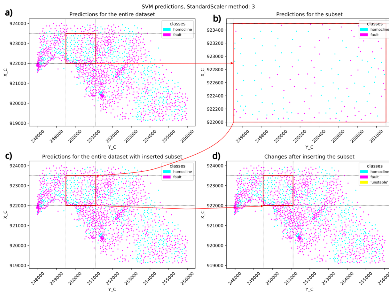
Fig. 10 Results for the classification task for real data using Method 3: “Canonical ML scaling” as presented in the Methods section: (a) predictions for the entire dataset; we marked a subset using a red rectangle for further analyses in the next panels. (b) a subset from the entire dataset was selected for the classification task and the results are presented accordingly; (c) the results here are equivalent to those presented in panel (a). (d) this panel shows that the set corresponding to “unstable” observations is an empty set due to common transformation parameters for training, test and real data.
