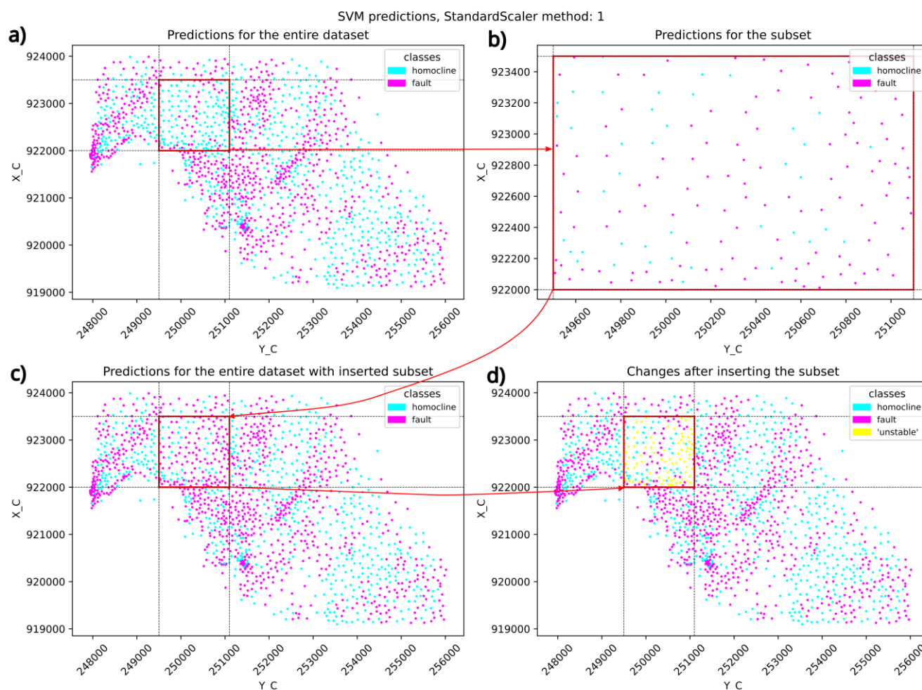
Fig. 8 Results for the classification task for real data using Method 1: “Independent subset scaling” as presented in the Methods section: (a) predictions for the entire dataset; we marked a subset using a red rectangle for further analyses in the next panels. (b) a subset from the entire dataset was selected for the classification task and the classification results are presented accordingly; (c) the results here are equivalent to those presented on panel (a) except the area marked with a red rectangle. In this area, we inserted the results from panel (b). (d) to better observe spatial continuity of the results, we marked discrepancies in the classification results using yellow labels.
