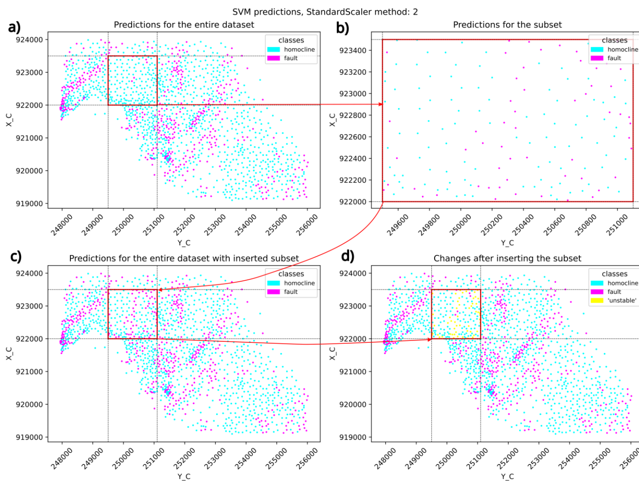
Fig. 9 Results for the classification task for real data using Method 2: “Per-surface local scaling” as presented in the Methods section: (a) predictions for the entire dataset; we marked a subset using a red rectangle for further analyses in the next panels. (b) a subset from the entire dataset was selected for the classification task and the classification results are presented accordingly; (c) the results here are equivalent to those presented on panel (a) except the area marked with a red triangle. In this area, we inserted the results from panel (b). (d) to better observe dependence of the classification results on the area taken for the analysis, we marked discrepancies in the classification results using yellow labels.
