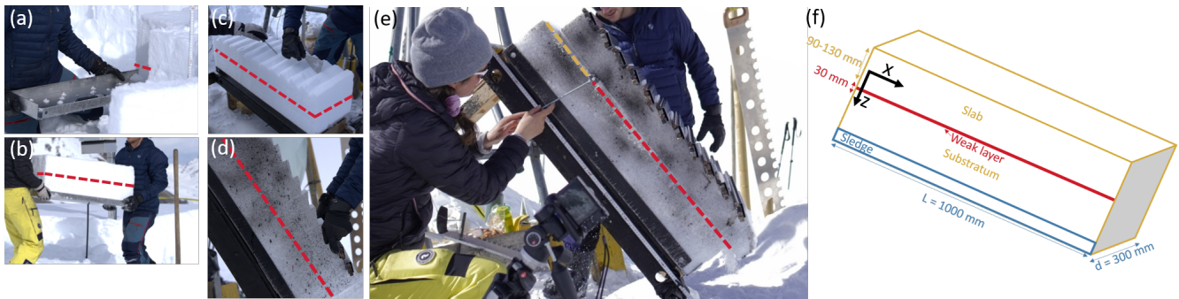
Figure 3. a) and b) Extraction of the sample using the sledge, with the weak layer highlighted by the red dashed line. c) Preparation of the sample by creating stair-step notches in the slab. d) Close-up of the stair-step notches in the slab and the weights that are placed in these notches. e) MMFT setup, including the weights on top of the slab and a camera in front of the setup. Captured is the moment just after the critical cut length was reached (indicated by the yellow dotted line), when the crack propagates through the weak layer and the slab has already started to slide down. f) Schematic overview of the MMFT setup: the weak layer is highlighted in red. Below the weak layer is the substratum, placed on top of the aluminum sledge.
