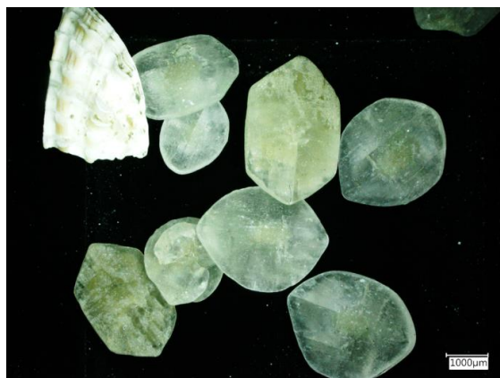
685 Figure A1: Authigenic crystals from sample S45 (grain size fraction >2000 μm) identified as gypsum.
