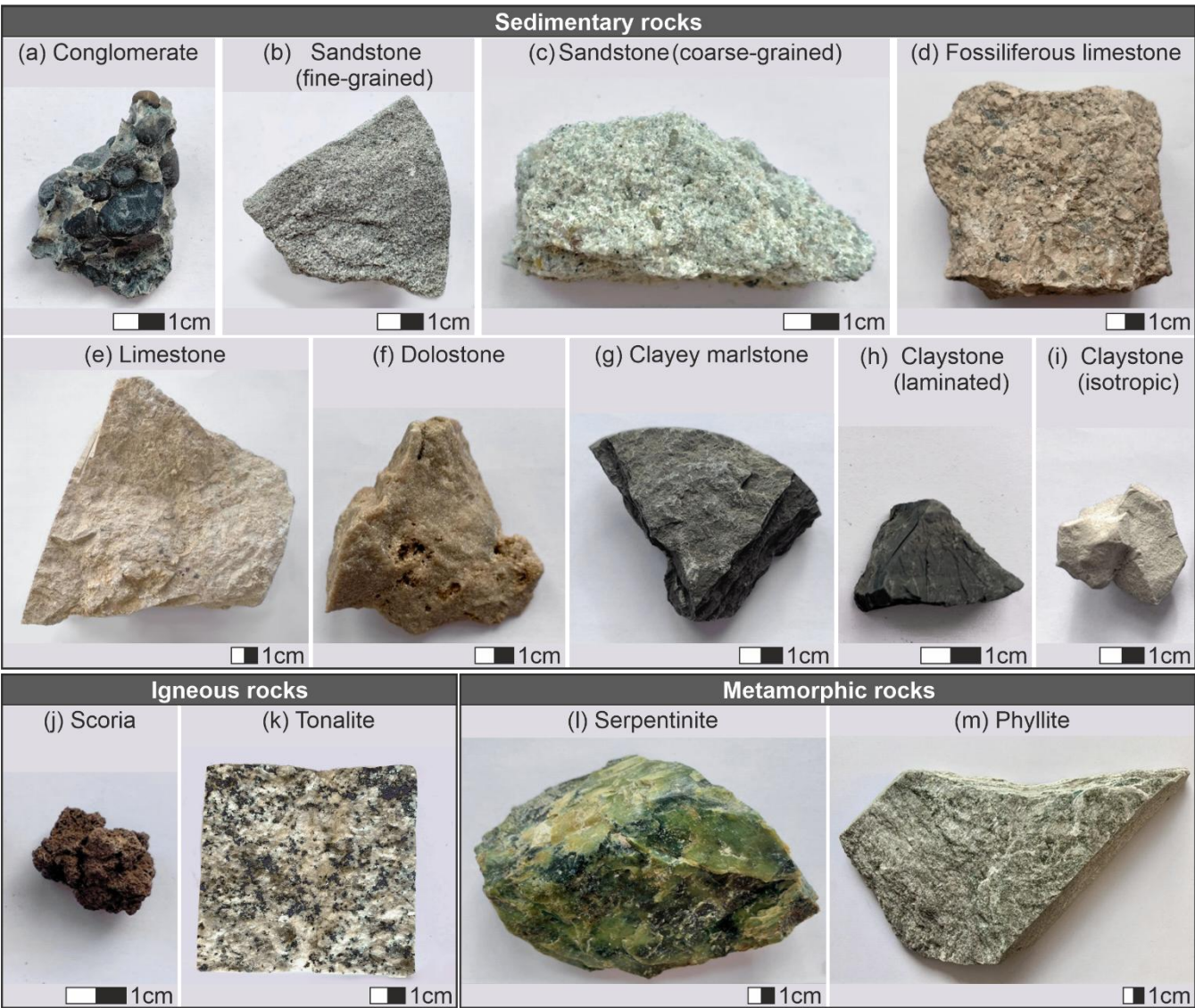
Figure 4: Tested rock samples and related rock categories. Top row: (a) conglomerate, (b) fine-grained sandstone, (c) coarse-grained sandstone, (d) fossiliferous limestone. Middle row: (e) limestone, (f) dolostone, (g) clayey marlstone, (h) laminated claystone, and (i) isotropic claystone. Bottom row: (j) scoria, (k) tonalite, (l) serpentinite, and (m) phyllite.
