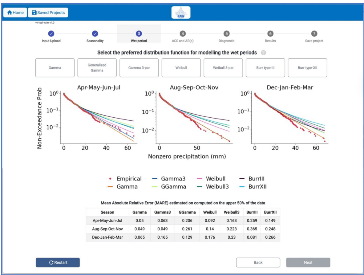
Figure A.4: Wet period module: calibration results of marginal distributions for non-zero rainfall values.
