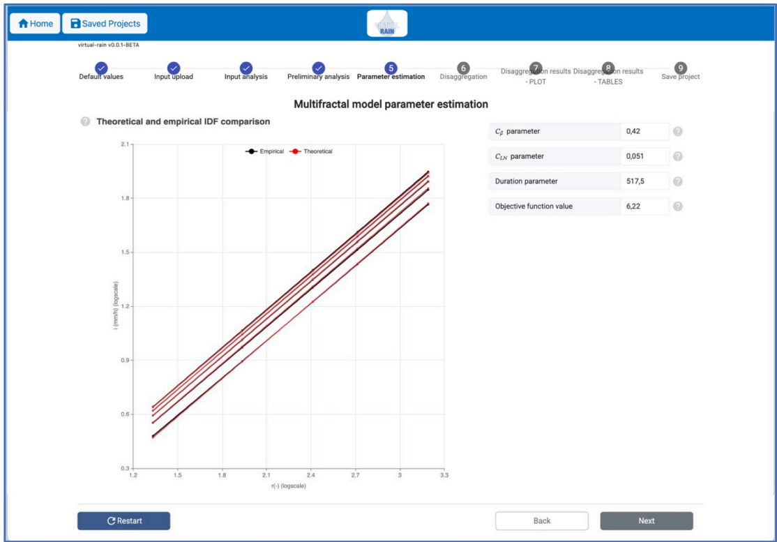
545 Figure A.11: MRC calibration interface showing the comparison between imposed and calibrated IDF curves for the selected return periods, together with the estimated MRC parameters and objective-function value.
