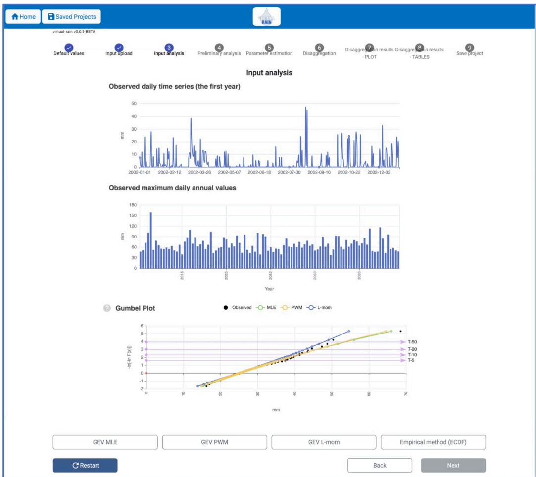
Figure A.9: Preliminary analysis interface showing daily rainfall for the first year, annual maximum daily rainfall and the Gumbel plot comparing GEV fits obtained through MLE, PWM and L-mom methods.
