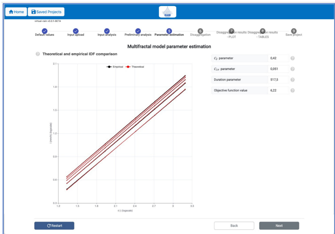
735 Figure A.11: MRC calibration interface showing the comparison between imposed and calibrated IDF curves for the selected return periods, together with the estimated MRC parameters and objective-function value.
