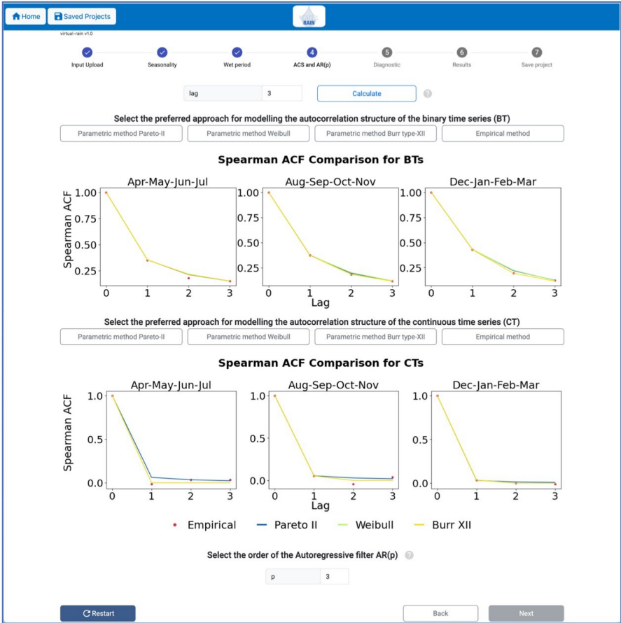
Figure A.5: ACS and AR(p) interface: calibration results of the autocorrelation structure.
