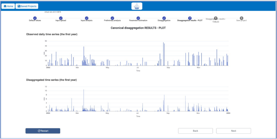
Figure A.13: Disaggregation results interface showing the comparison between the observed daily rainfall series and the generated sub-hourly disaggregated series for the first simulation year.
