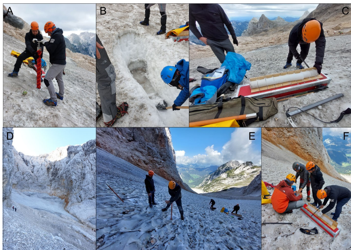
Figure S3. Sampling approach at Triglav Glacier (A-C) and Skuta Glacier (D-E). A – Start of ice coring from the snow-covered ice mass at Triglav Glacier. B – Laterally dug trench to bypass the rocky layer at 0.9-1.0 m. Note that the stratigraphy of the trench, with top 10 cm represented by snow, bracketed by dust layers on top and below it, followed by firn ice down to a depth of ~70 cm, and ice further down, with a rocky layer at depth of 0.9-1.0 m. C – Subsampling by cutting the ice core in 10 cm-long sections. Note the open topography around Triglav Glacier.
